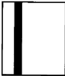
Vertical black streaks Refer to RAP 11 Refer to RAP 15
